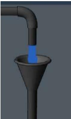
An air gap prevents the reverse flow of water. The gap should be at least twice the pipe diameter but not less than 25 mm. There should also be an overflow with a capacity of at least the inflow capacity.
