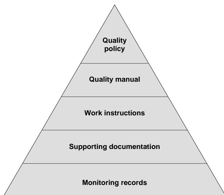
Figure 2.7: Basic structure for a quality management system
