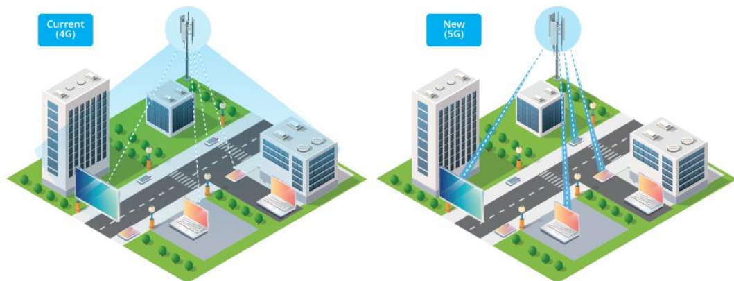
Figure 1: Conventional antenna (left), and beam-forming antenna (right)
