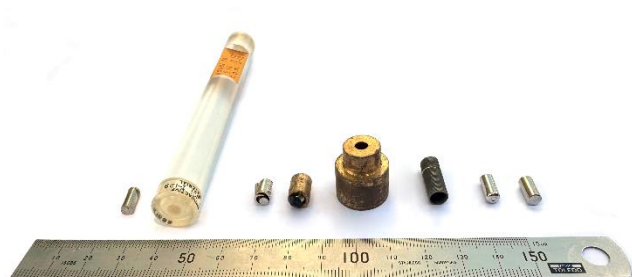
Figure 6: Various radioactive sources typically used in most of the applications described above. Maximum length about 3 cm. Maximum diameter about 0.5 cm.
