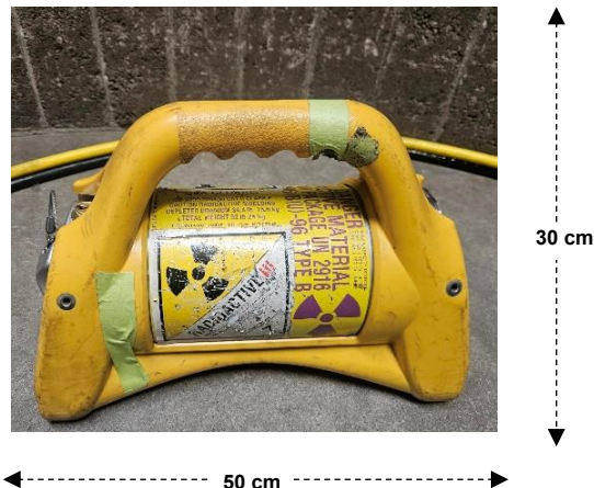
Figure 5: Shielded radioactive device used in transporting and operating industrial gamma radiography systems, such as for weld inspections in engineering and construction.
