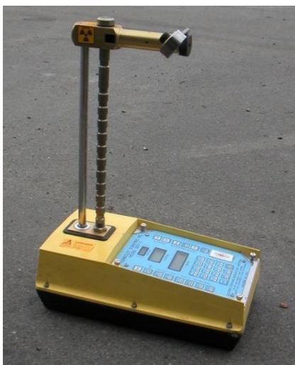
Figure 8: Moisture density gauge used in road building and agriculture.
