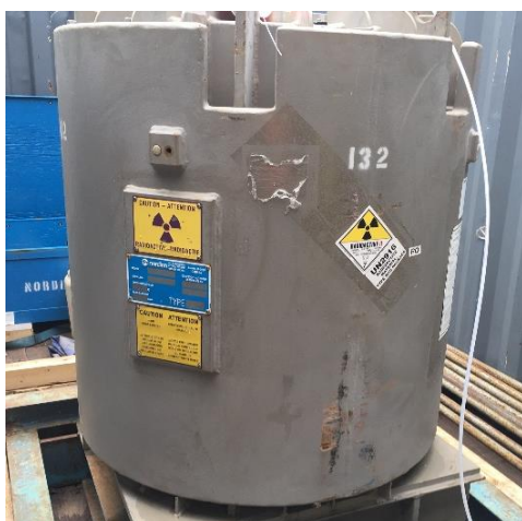
Figure 2: Shielded package used for transporting high-strength radioactive sources for industrial irradiation.
