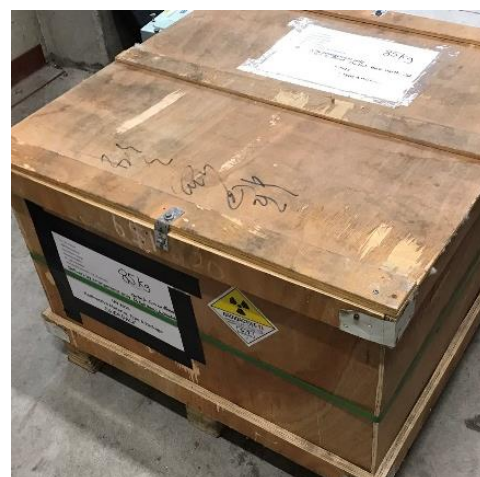
Figure 3: Package used for transporting a gauging system loaded with radioactive sources.
