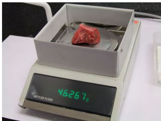
Figure A2-2: Photographs of the equipment used for the measurement of density. The balance on the left was used to measure the weight of a sample in air and the cage shown in the photograph on the right was slung from below this scale and used to weigh the sample underwater at < 6^{\circ}\text{C} . The bowl was filled with 3 litres of chilled, de-bubbled (by boiling), RO water.
