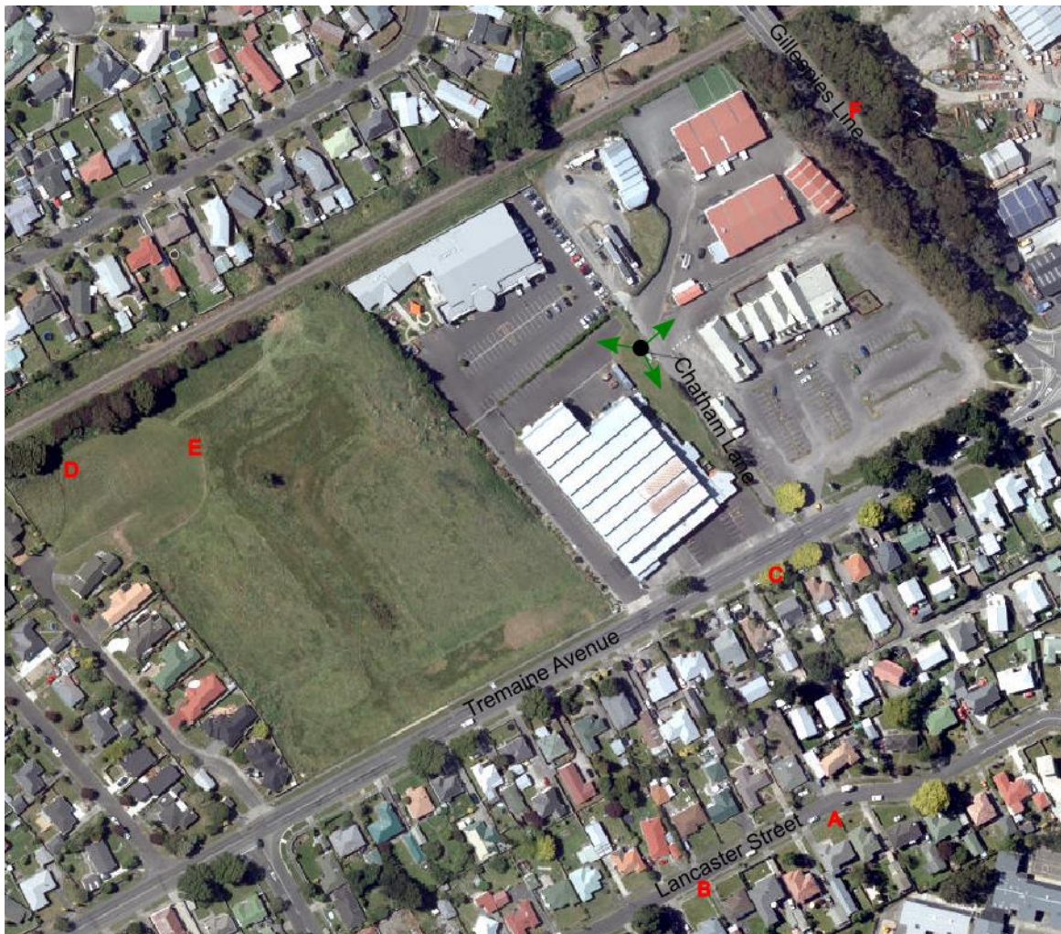
Fig 9. Measurement locations near the Cloverlea site. Letters in red show where measurements were made. Green arrows show the orientations of the antennas at the Spark site.
