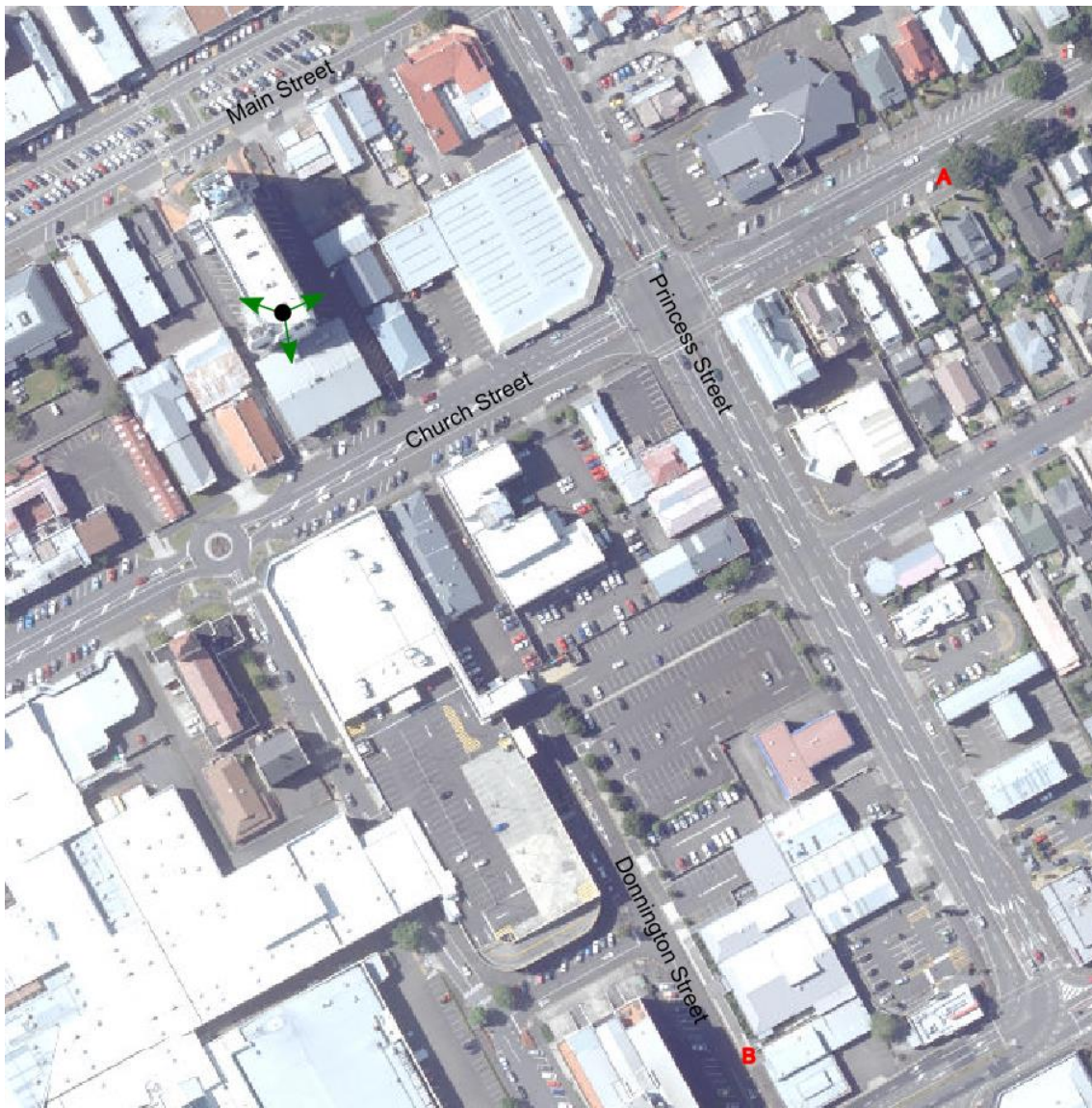
Fig 18. Measurement locations near the Palmerston North site. Letters in red show where measurements were made. Green arrows show the orientations of the antennas at the Spark site.
