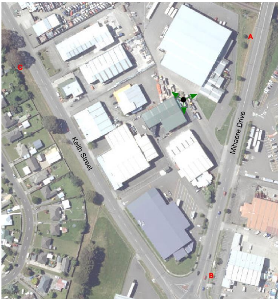
Fig 24. Measurement locations near the Terrace End site. Letters in red show where measurements were made. Green arrows show the orientations of the antennas at the Spark site.
