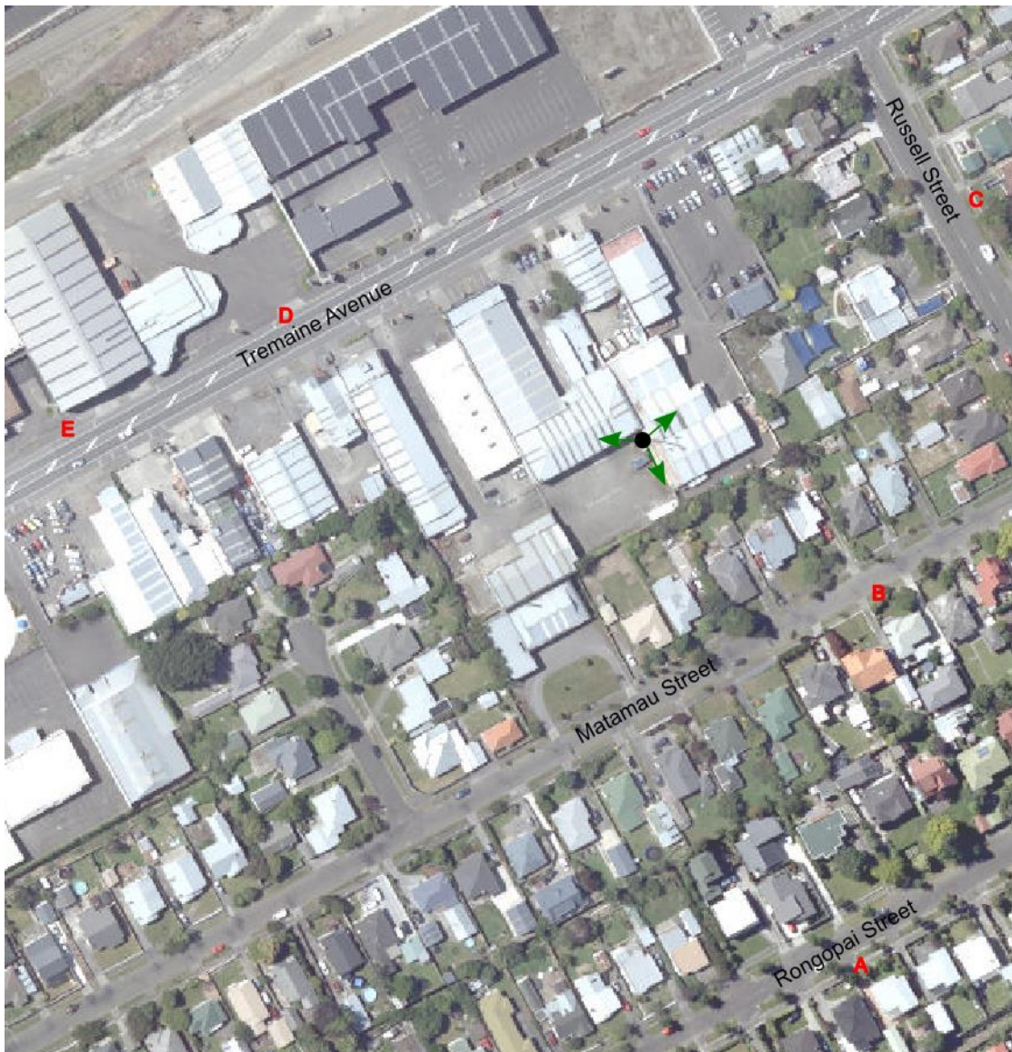
Fig 15. Measurement locations near the Papaioea site. Letters in red show where measurements were made. Green arrows show the orientations of the antennas at the Spark site.
